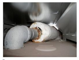
shall specify Elster Perfection Clearflow<sup>©</sup> Dielectric Waterway Fittings (or equivalent), which separate dissimilar metals in the electrolyte (waterway) - reducing the local galvanic cell.
